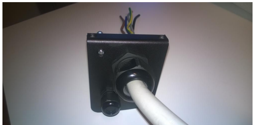
Figure 23: Power supply cable pulled through the gland – front view
