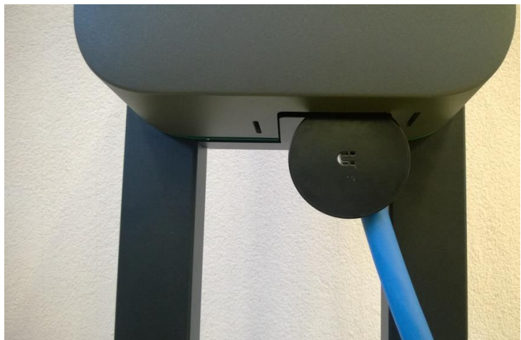
Figure 50: Charging station with the installed small metal circle where magnetic cable hand can be attached to
