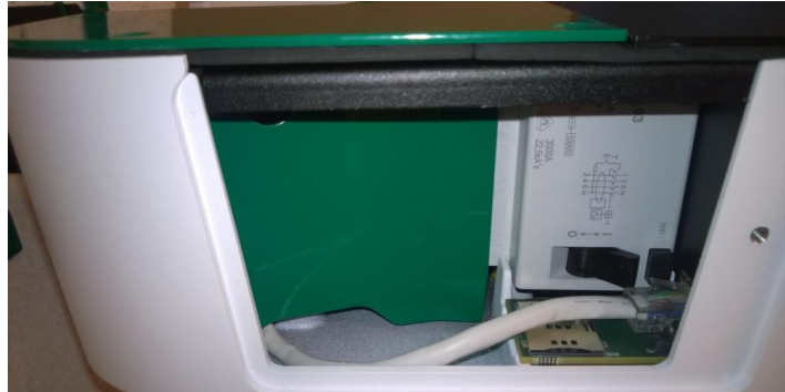
Figure 43: Side view of the reattached back maintenance door
