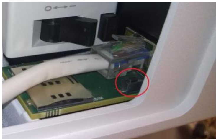
Figure 20: Charging station reset button
