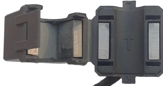
Figure 12: Arrow pointing in the direction of energy flow
