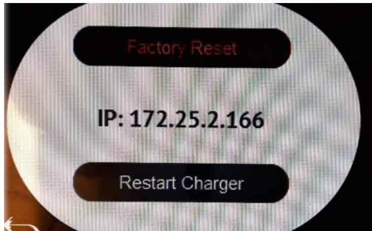
Figure 21: Display of IP address after pressing the reset button for 5 s
