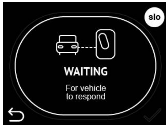
Figure 17: Charging station is waiting for EV to responds and starts charging
