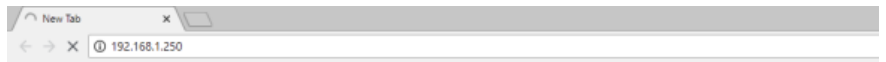
Figure 20: Insert the default IP into the browser to connect to web interface
