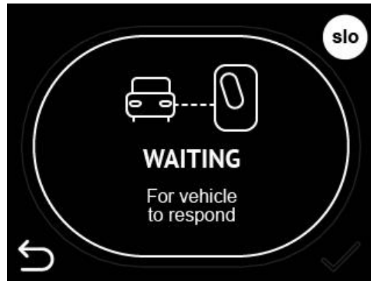
Figure 15: Charging station is waiting for EV to responds and starts charging
