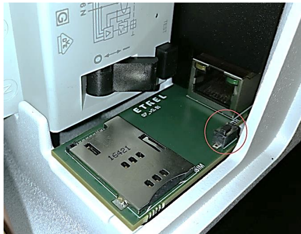
Figure 40: Reset button inside the maintenance opening
