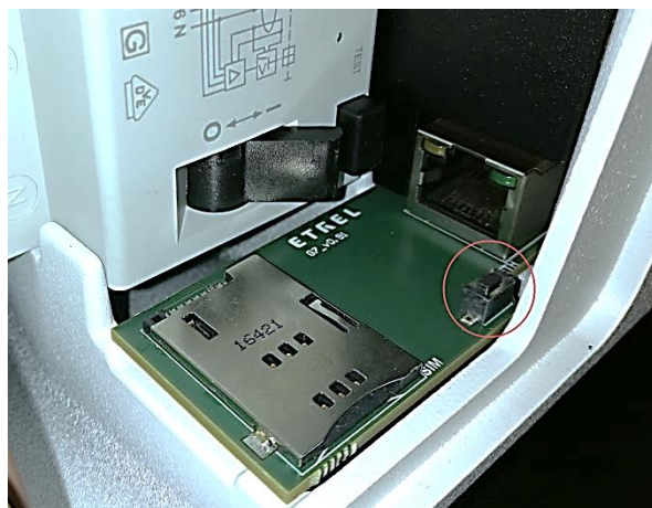
Figure 37: Reset button inside the maintenance opening
