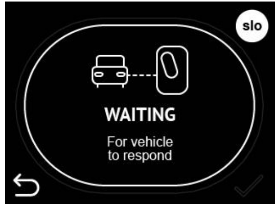
Figure 12: Charging station is waiting for EV to responds and starts charging
