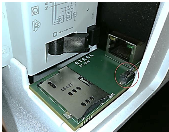
Figure 37: Reset button inside the maintenance opening
