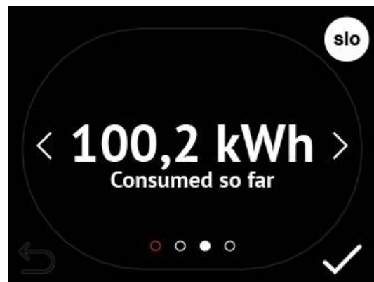
Figure 14: Example of shown energy on the LCD screen
