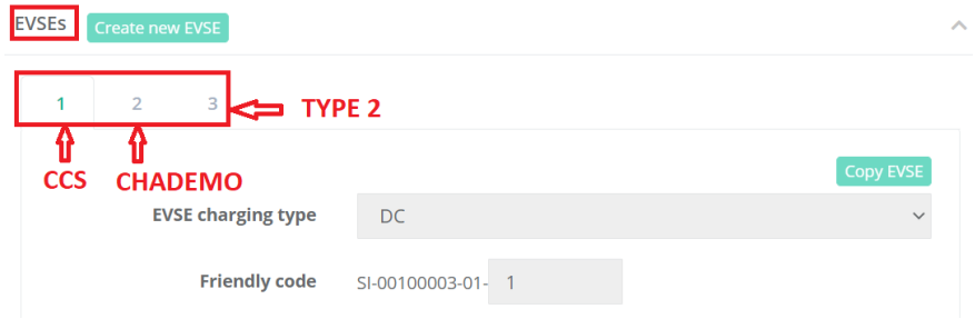
Figure 4: A setup of roaming DC charging station. It has three EVSEs, each having one connector. The first EVSE has CCS connector, the second EVSE has Chademo connector and the third EVSE has a type 2 connector.
