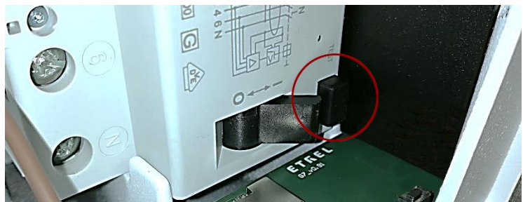
Figure 11: RCD test button
