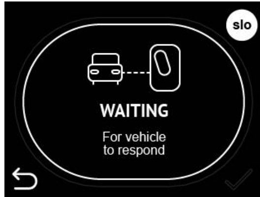
Figure 7: Charging station is waiting for EV to respond and starts charging
