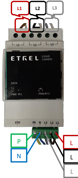
Figure 10: Arrangement of input and output phases
