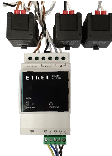
Figure 5: Load Guard with connected measuring current transformers
