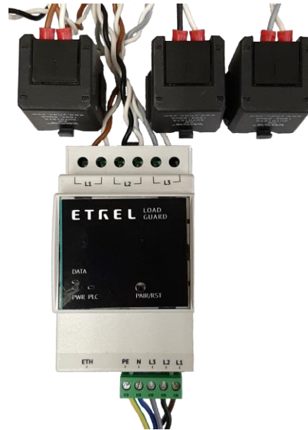
Figure 5: Load Guard with connected measuring current transformers
